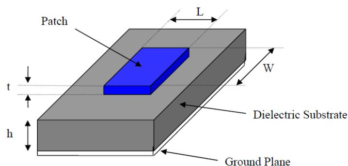
Fig. 1: Configuration of a microstrip antenna
